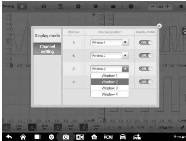
Figure 7-33 Sample Channel Setting Screen
